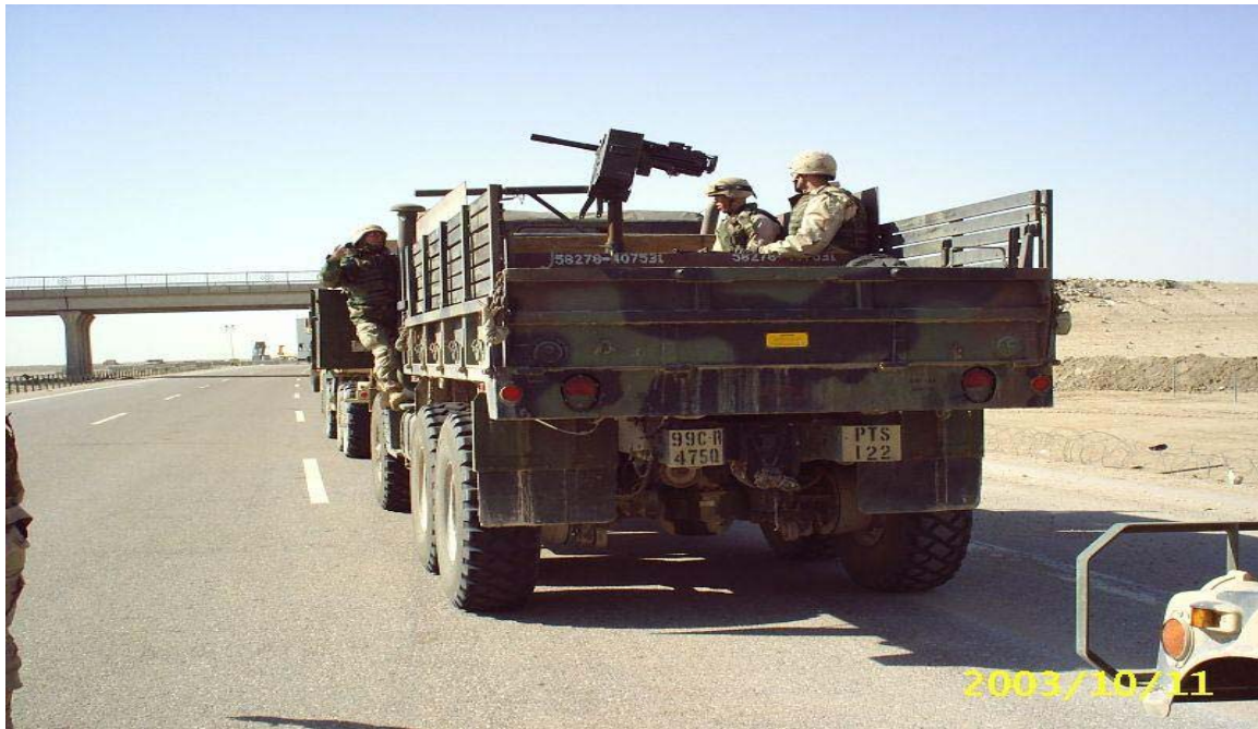
Figure 6-4. Armor Plating Surrounding the Gun Platform
